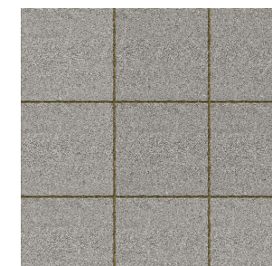
Courtyard Walkway 0.6m x 0.6m Concrete Pavers
